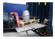
However, an address on his route was incorrect and the order of 12 beer kegs was undeliverable. The worker was moving the kegs with a pallet truck to access the next load when he fell from the raised tail lift on to the road. Several kegs of beer fell and struck him, resulting in a traumatic brain injury and facial fractures that required metal plates to be inserted into his skull.
